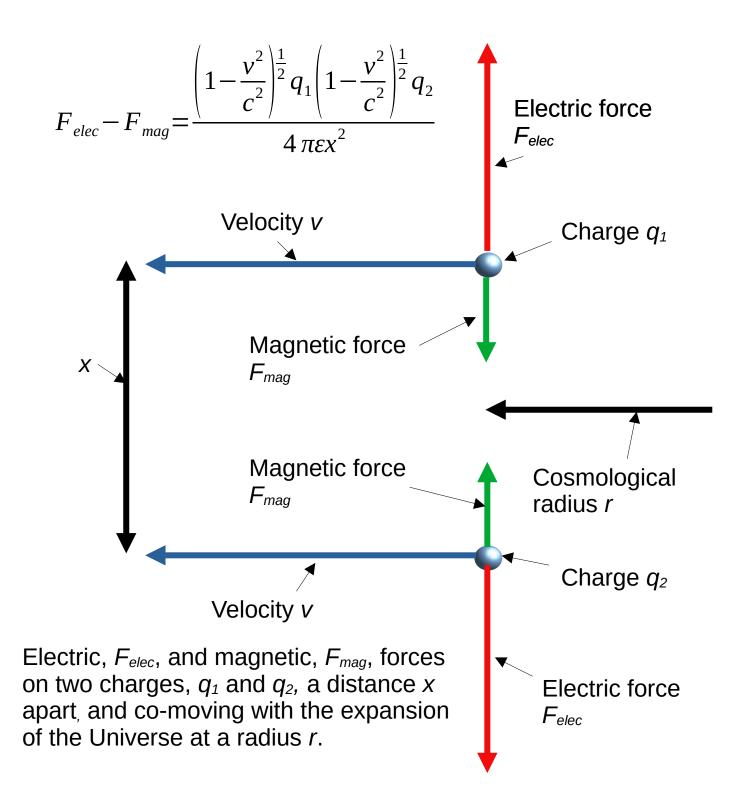
As the velocity, v, approaches the speed of light, c, the resultant force,  $F_{elec} - F_{mag}$ , tends to zero
